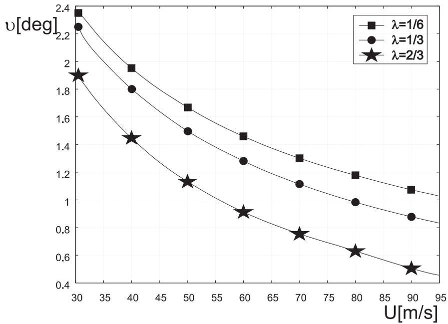
**Figure 14** Influence of dimensionless LCG  $\tilde{\xi}$  on stability
