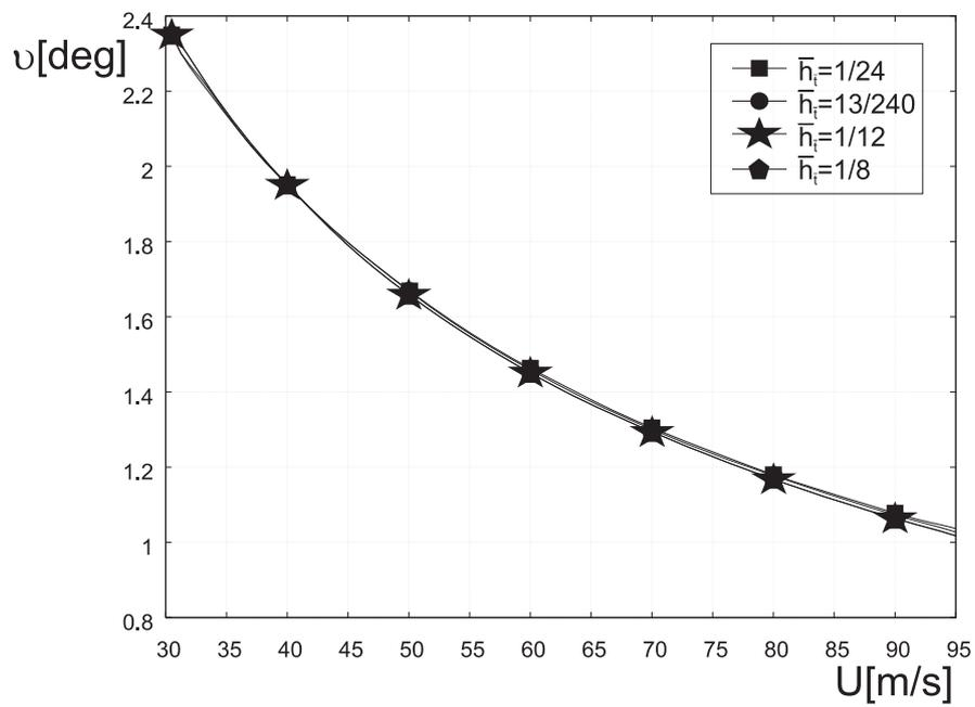
Figure 12 Influence of dimensionless mass moment of inertia  $i_z$  on stability
