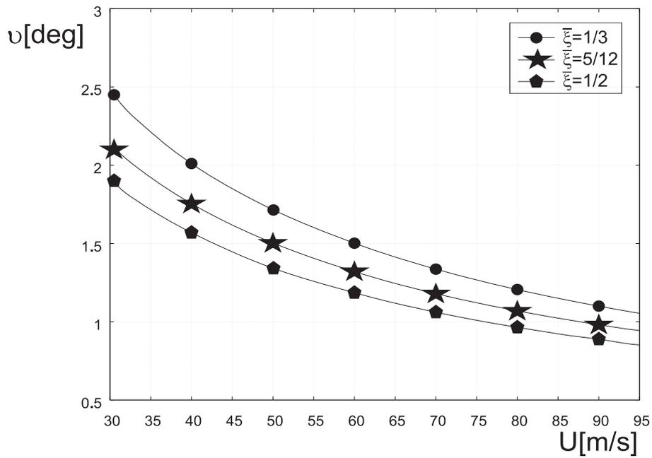
**Figure 10** Influence of dimensionless vertical centre of gravity  $\tilde{\eta}$  on stability
