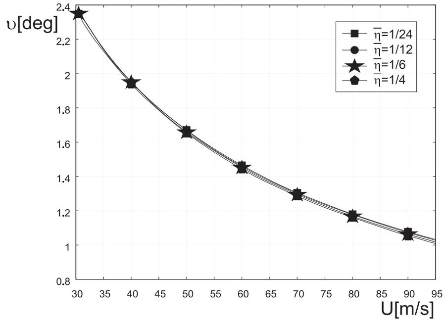
**Figure 11** Influence of dimensionless height of the boat at transom  $\tilde{h}_t$  on stability
