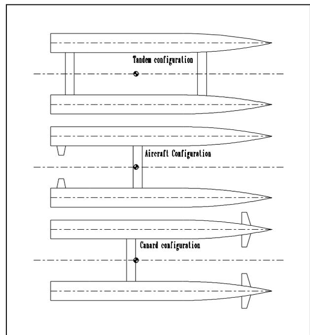
**Figure 14: Hydrofoil Configurations**
