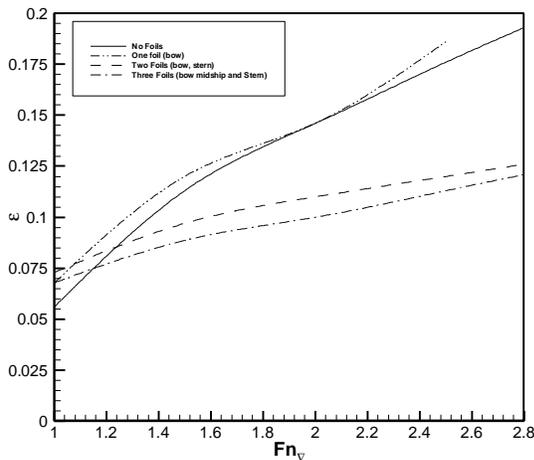
**Figure 4: Resistance Comparisons for planing catamarans with tandem foils**
