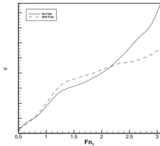
**Figure 3: Resistance Comparison for a Semi-Displacement Catamaran**
