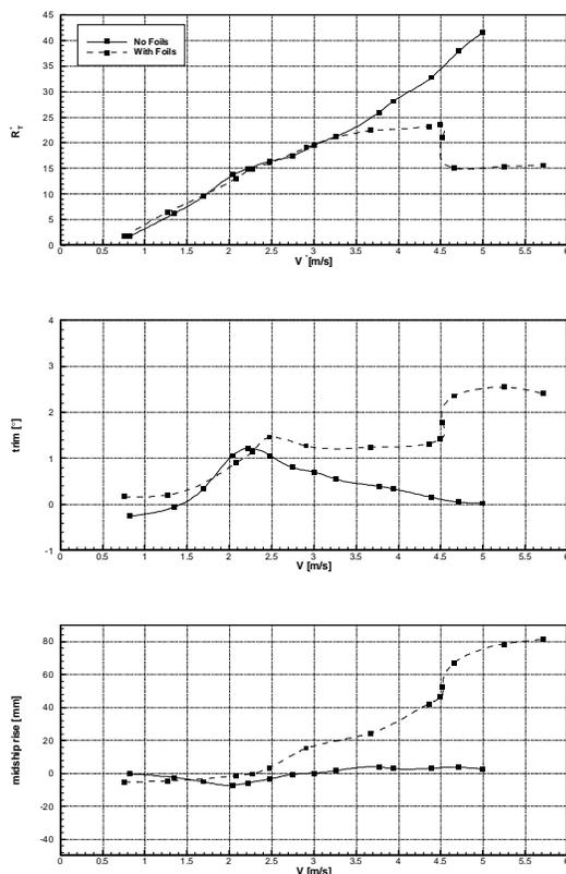
**Figure 16: Changes in Resistance, trim and sinkage due to unloading of hull**
