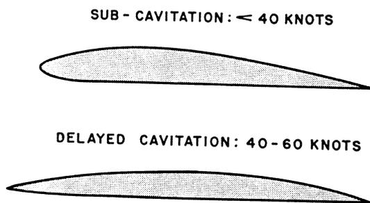
**Figure 13: Sub-Cavitation section compared with Delayed Cavitation section**
