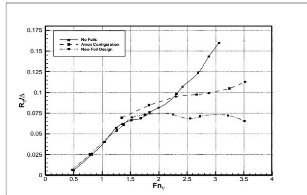
**Figure 18: Resistance tendencies for a 40m semi-displacement vessel with a new foil Arrangement**
