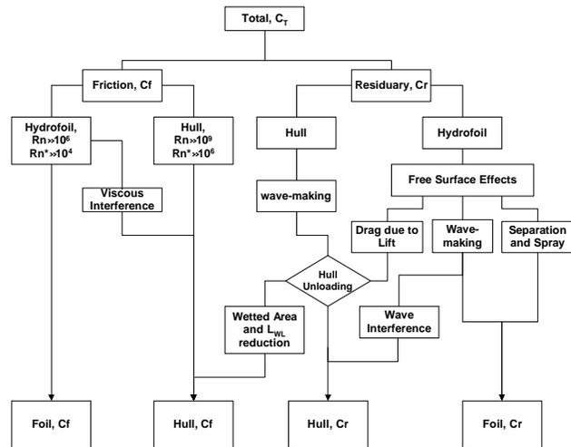
Figure 12: Resistance Breakdown for Hydrofoil Assisted Craft
