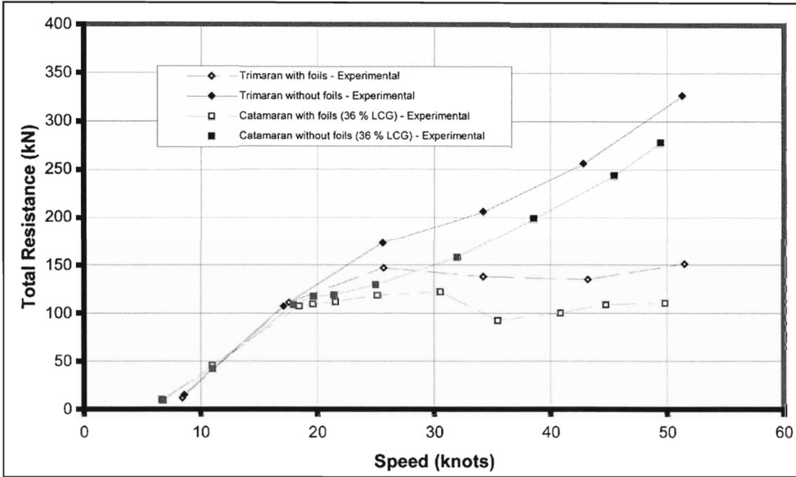
Figure 5: Total resistance vs speed for 32% LCG
