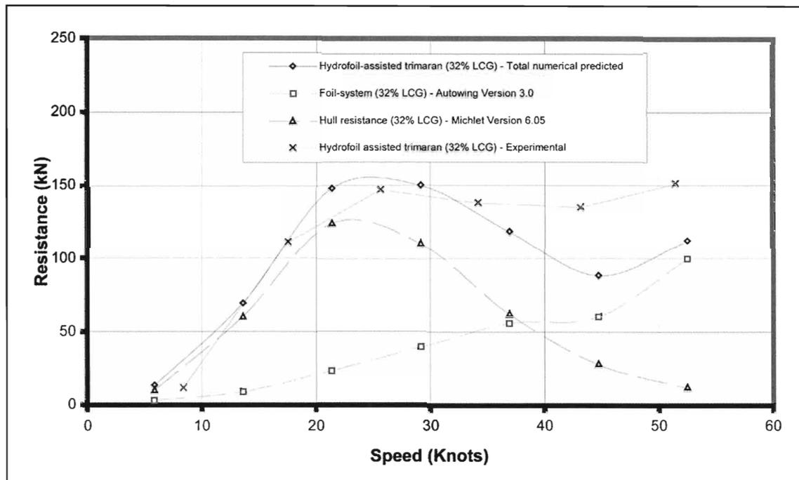
Figure 11: Resistance breakdown for 32% LCG position
