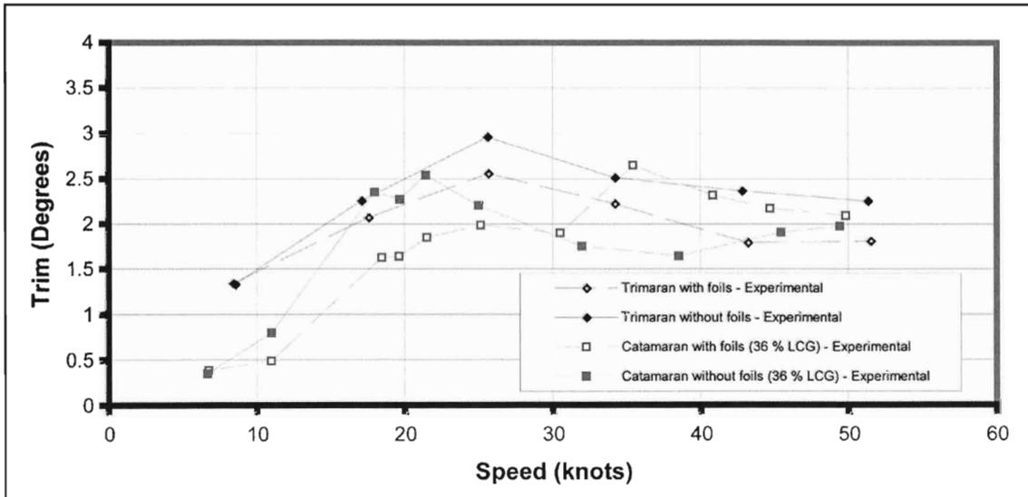
Figure 6: Trim vs speed for 32% LCG with foils compared to the catamaran
