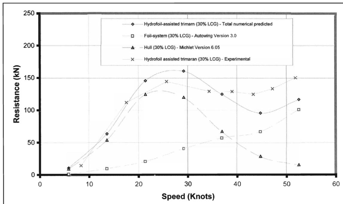
Figure 12: Resistance breakdown for 30% LCG position
