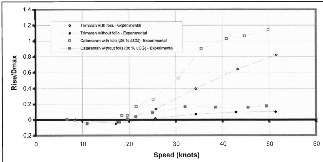
Figure 7: Rise-draft (maximum) ratio vs speed for 32% LCG with foils compared to the catamaran
