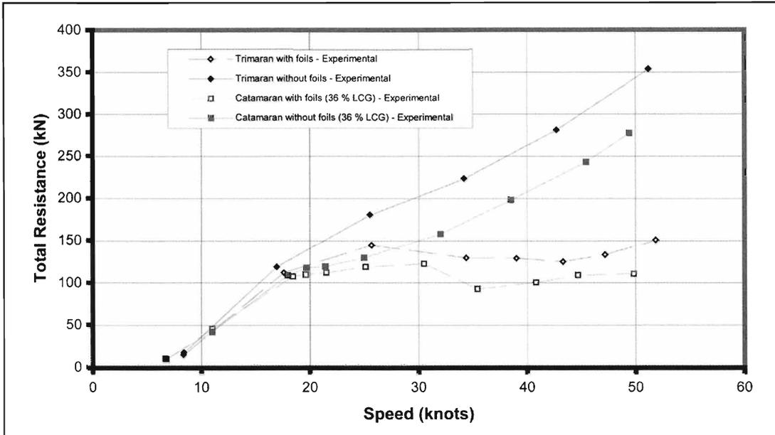
Figure 8: Total resistance vs speed for 30% LCG with foils compared to the catamaran
