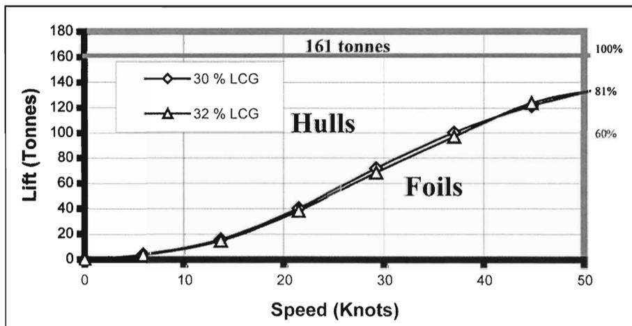
Figure 14: Load carried by foil system and hulls
