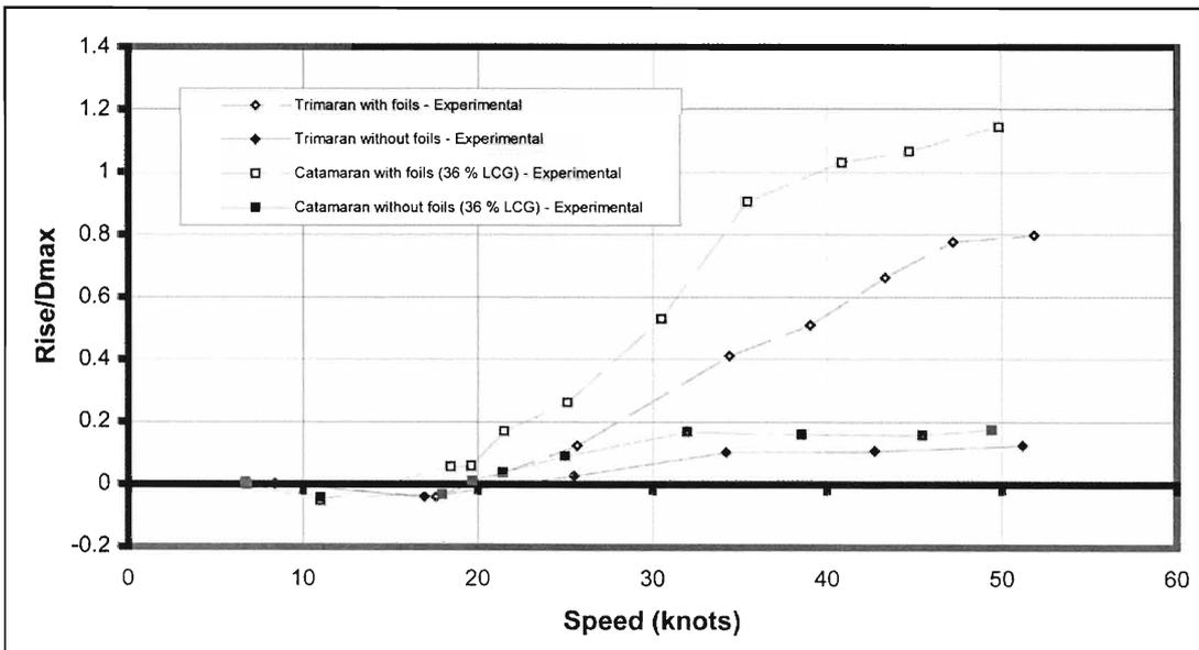
Figure 10: Rise-draft (maximum) ratio vs speed for 30% LCG with foils compared to the catamaran
