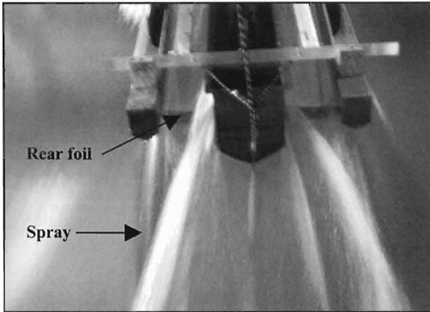
Figure 13: Significant spray caused by the rear foils at high speeds
